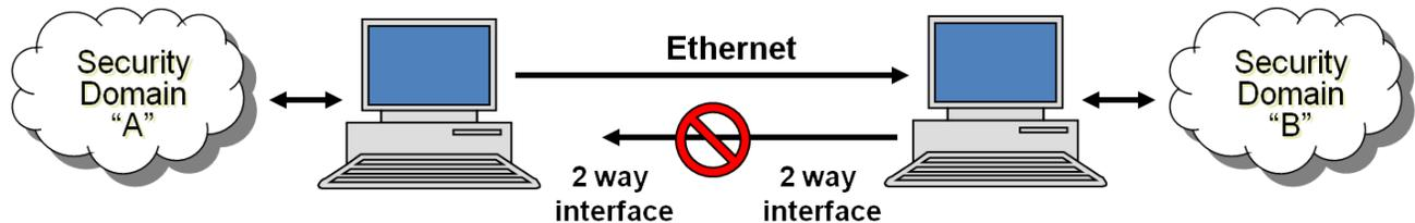
Figure 3: Ethernet Fakeout Method of Enforcing One-way Data Transfer
