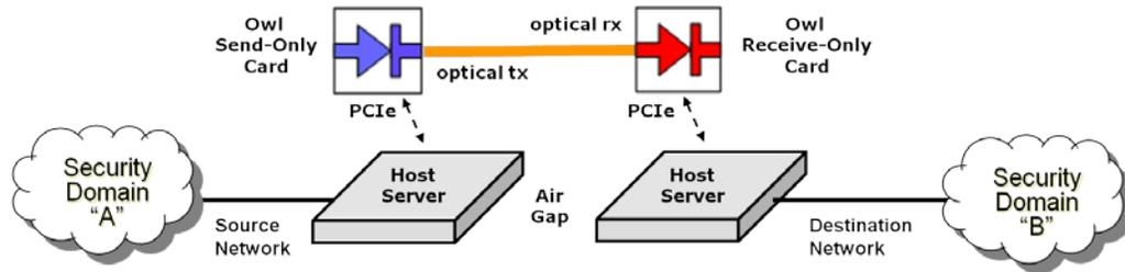
Figure 7: DualDiode Card Installation
