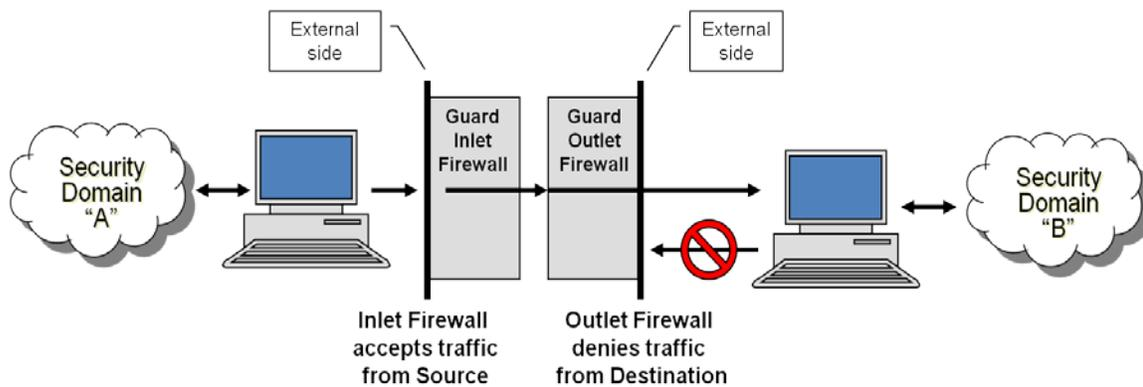
**Figure 6: Paired Firewalls Configured to Enforce One-Way Dataflow Policy**
