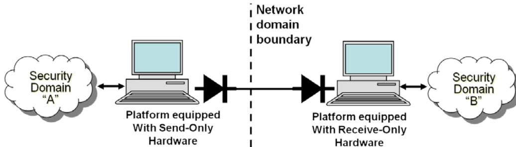
Figure 8: The DualDiode: One-Way Data Transfer Hardware at both Ends of Link
