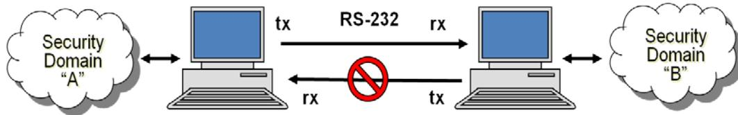
Figure 2: RS-232 with Modified Cable
