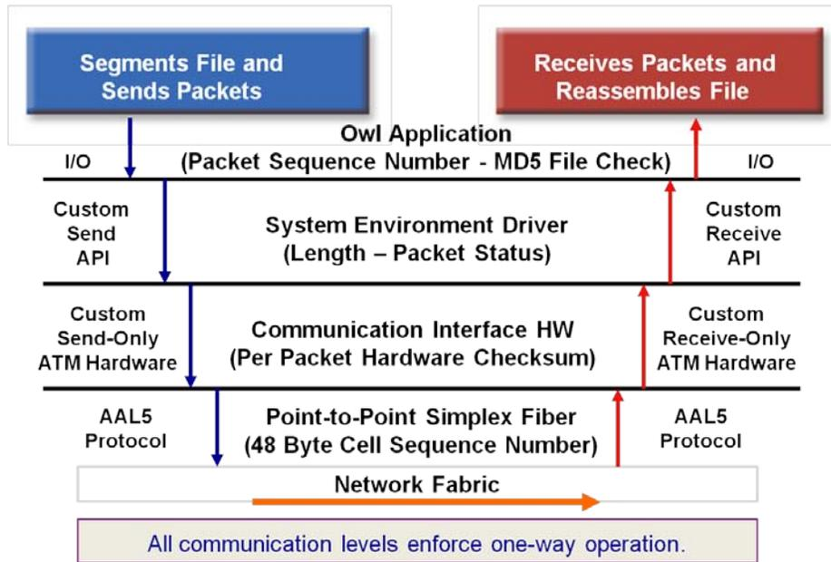
Figure 10: DualDiode Protocol Stack
