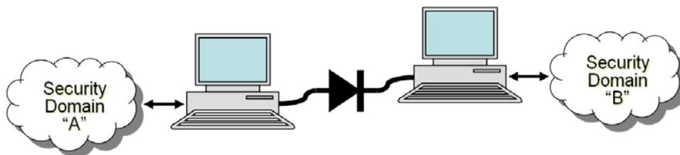
**Figure 1: Conceptual One-Way Interface between Networks**
