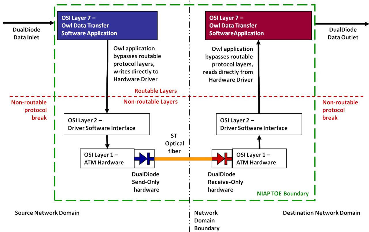
Figure 9: DualDiode Non-Routable Protocol Break
