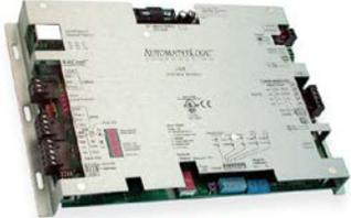
**1A-LGR:** Programmable controller with no analog inputs or outputs. Primary network is BACnet over Ethernet (not IP) media at 10/100 Mbps. Also supports BACnet over MS/TP media and proprietary protocol over RS-485 media. Can also be in Tier 2.
