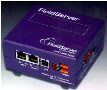
**3-FS:** A Tier 3 FPOC gateway (application layer proxy). The Tier 4 network is Modbus over IP over 10/100 Mbps Ethernet. The Tier 1 network is proprietary over proprietary 2-wire media. Note this is the same device as in 2C-FS.
