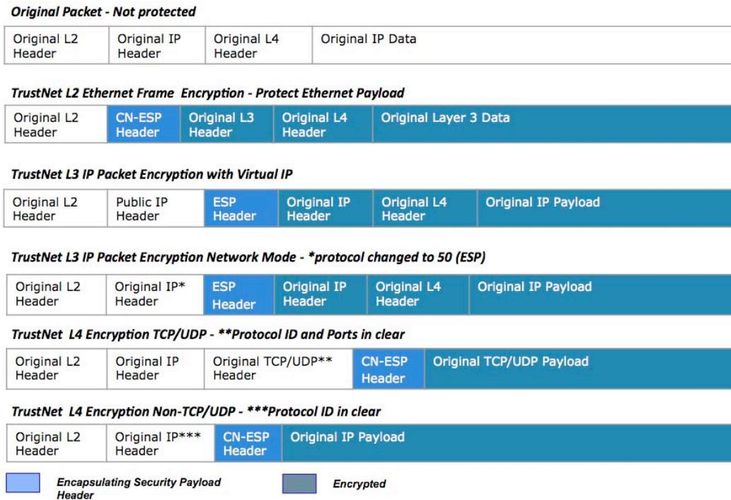
**Figure 3: TrustNet Packet and Frame Formats**
