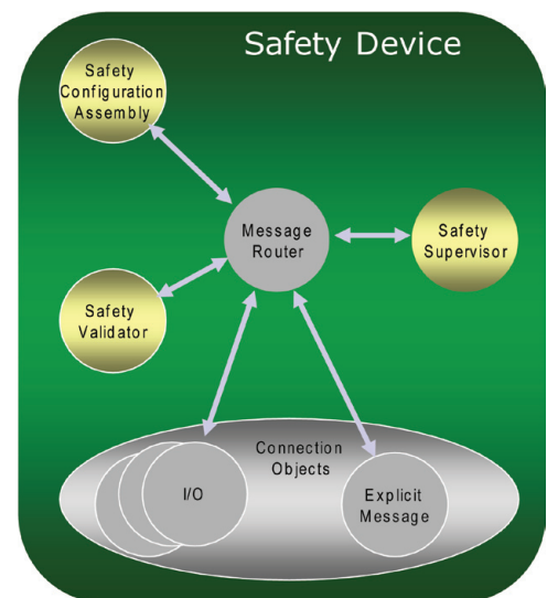
Figure 9 Configuring a safety device (Safety Supervisor)
