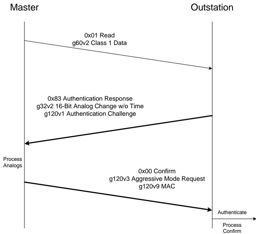
**Figure 7-26: Preventing Confirmation Challenge Collisions Using Aggressive Mode**
