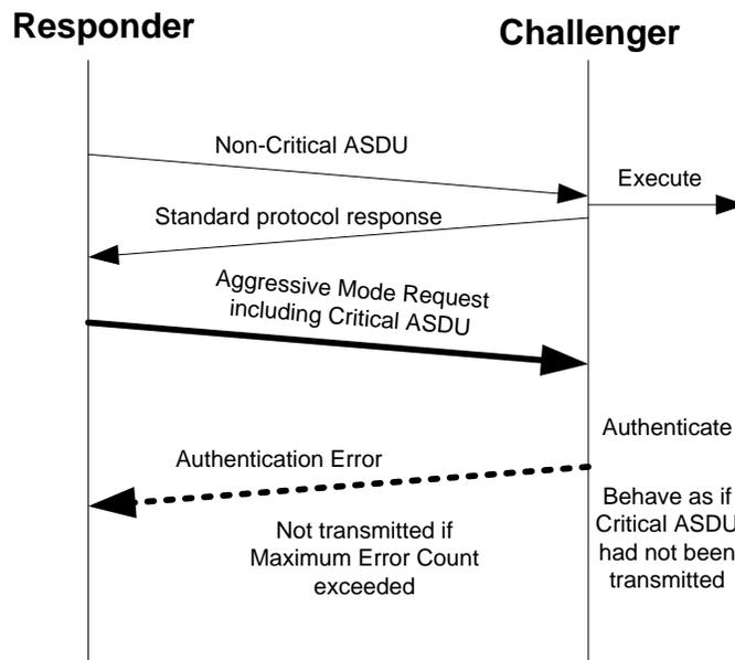
Figure 7-6: Example of a Failed Aggressive Mode Request
