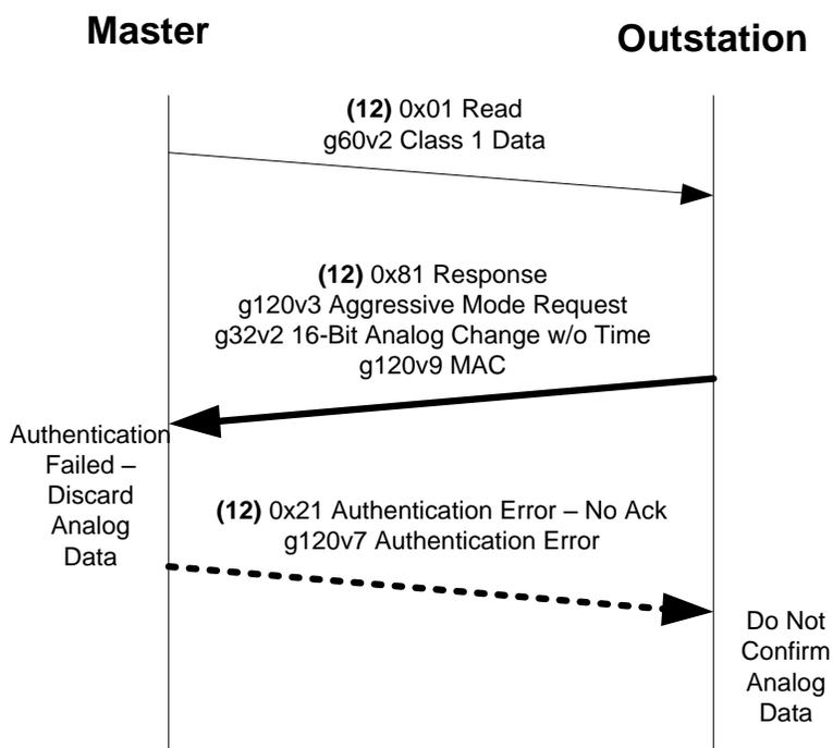
Figure 7-17: Example of Failed Authentication of Outstation Data
