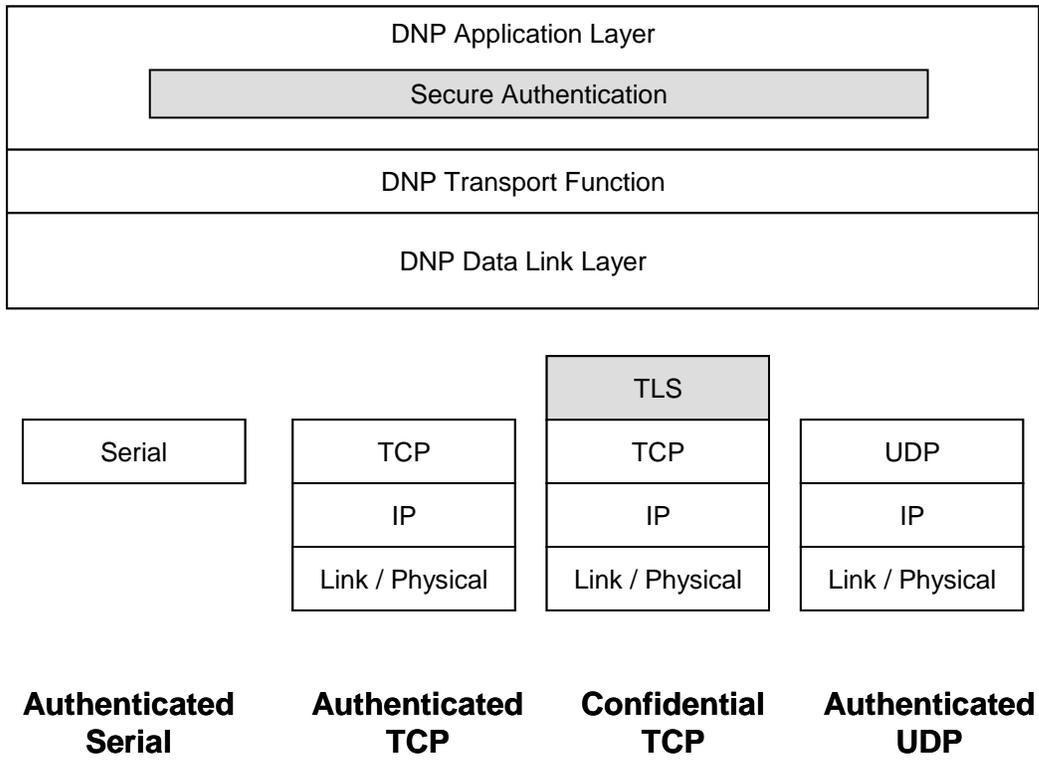
**Figure 7-30: Valid Profiles Using the Secure Authentication Mechanism**
