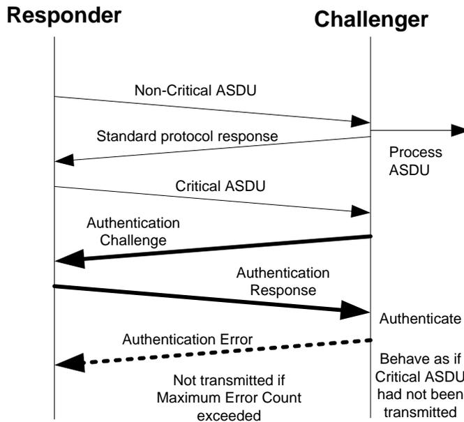
Figure 7-4: Example of Failed Challenge of Critical ASDU
