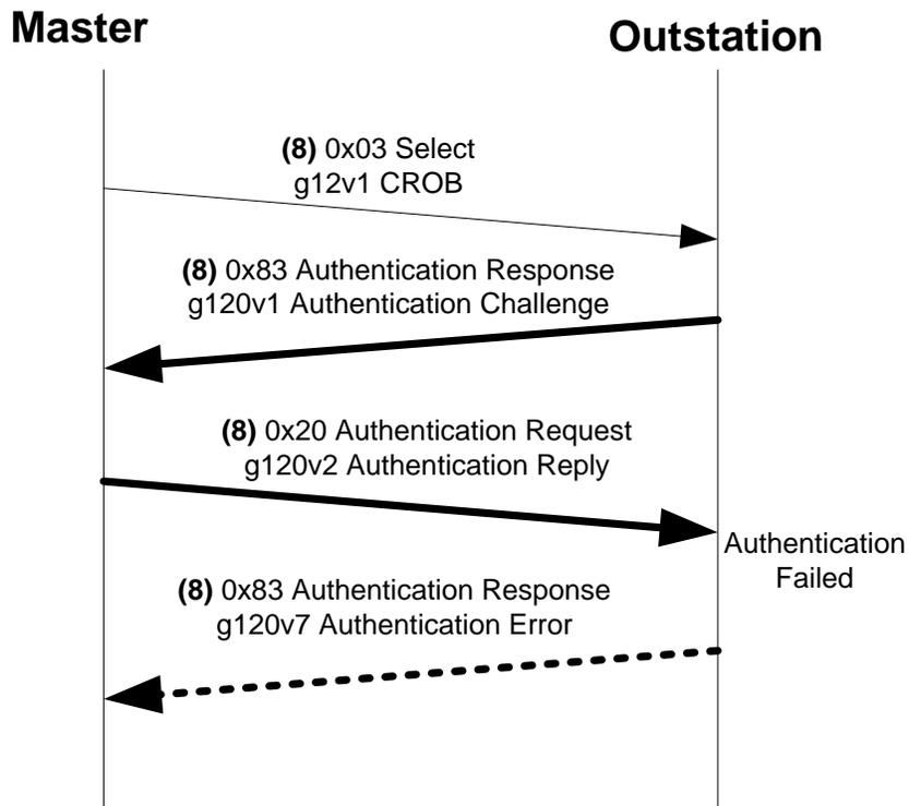
Figure 7-14: Example of Failed DNP3 Select/Operate Authentication
