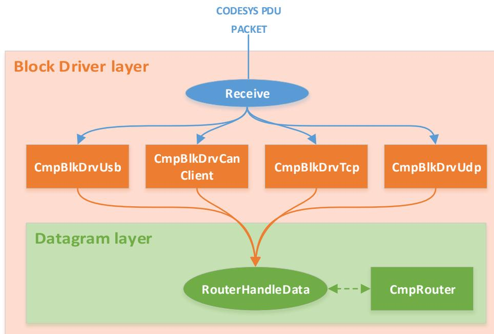
Schematic representation of how a CODESYS PDU packet is parsed by components at the Block Driver layer
