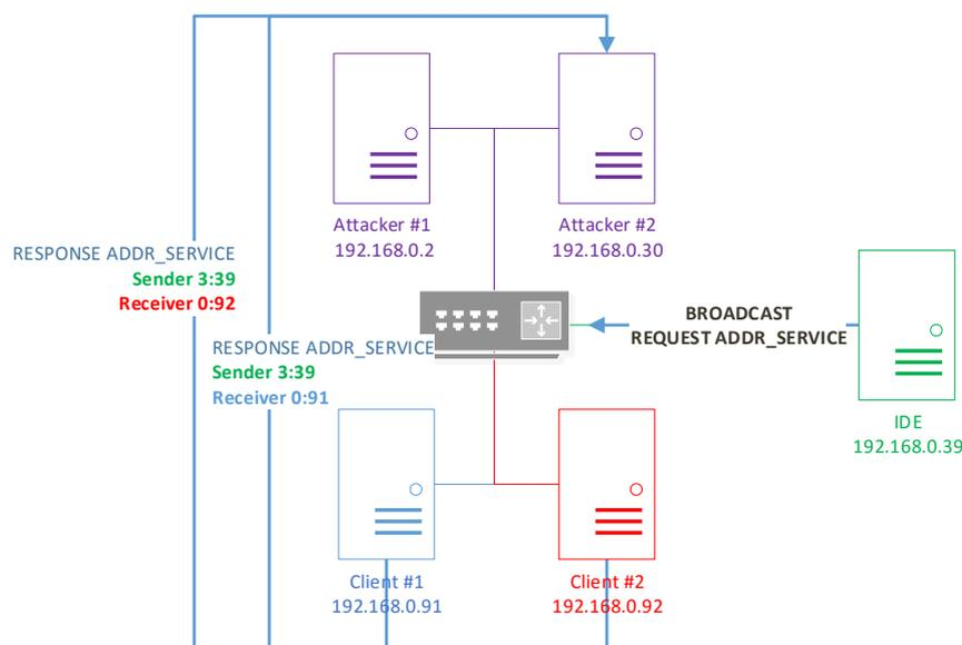
Schematic of a modified route of network traffic after setting an arbitrary parent node
