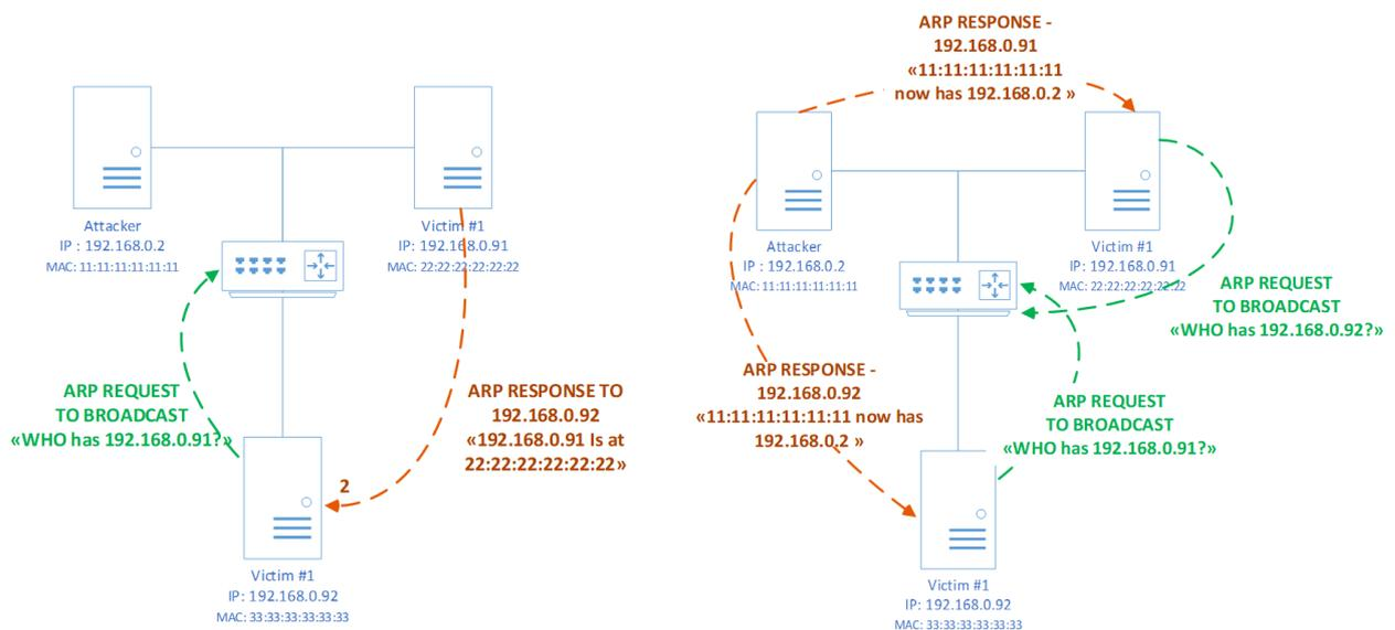
Schematic of an ARP poisoning attack over the ARP protocol. Step 1 is modification of the ARP table
