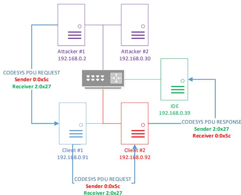
**Schematic of a modified IP spoofing attack over the CODESYS PDU protocol**
