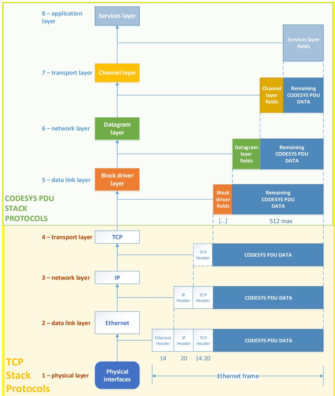
**Example use of the TCP and CODESYS PDU protocol stacks in one packet**
