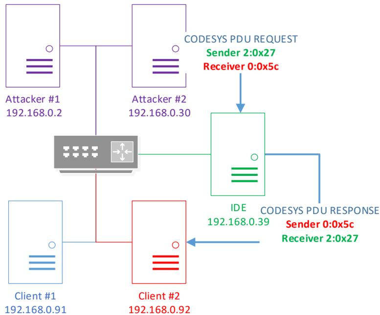
**Schematic of a classic IP spoofing attack over the CODESYS PDU protocol**
