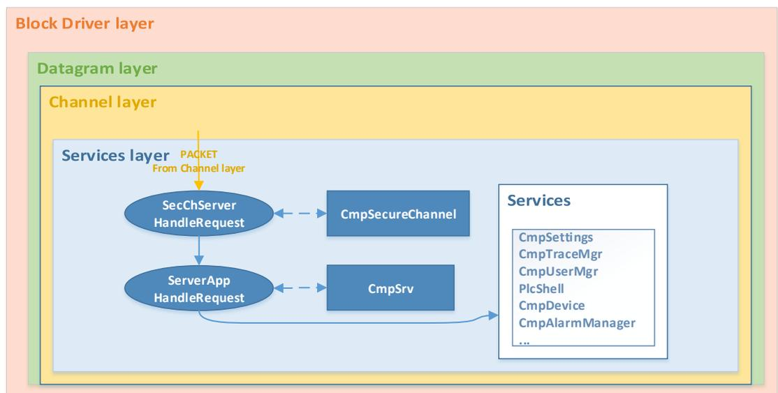
**Schematic representation of how a CODESYS PDU packet is parsed by components at the Services layer**
