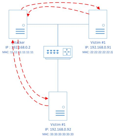
**Schematic of an ARP poisoning attack over the ARP protocol. Step 2 is the modified route of network traffic**
