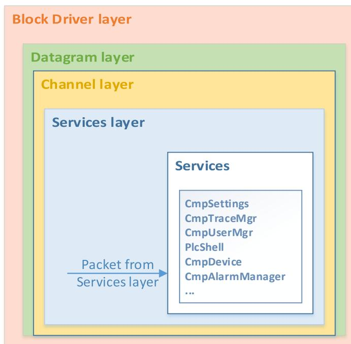
**Schematic representation of how a CODESYS PDU packet is parsed by components at the Services layer**
