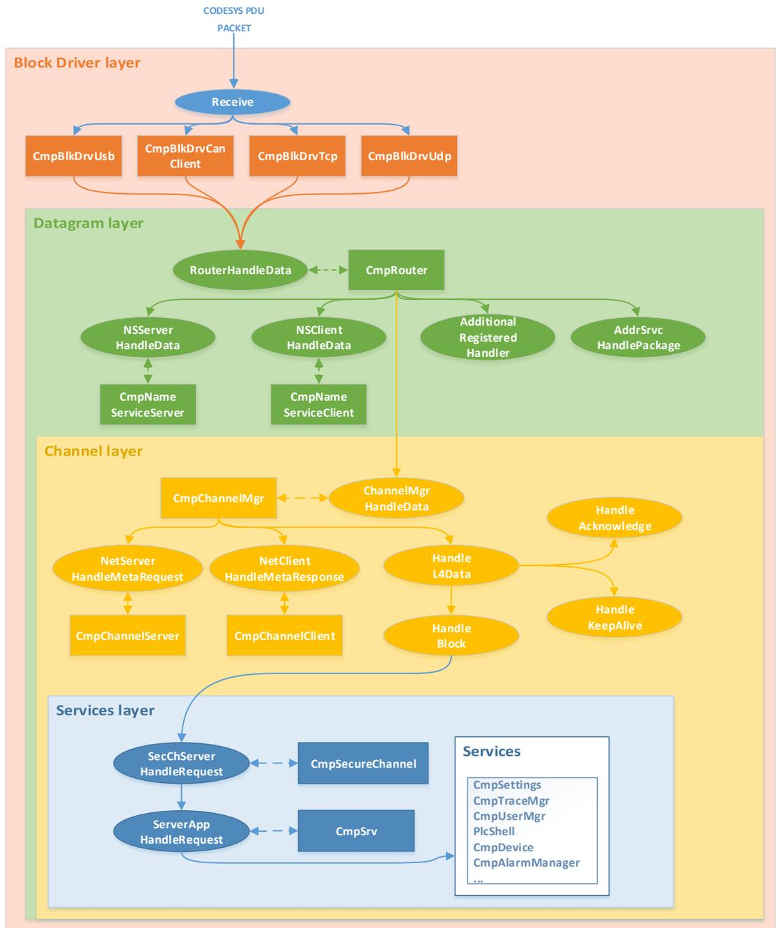
**Schematic representation of how a CODESYS PDU packet is parsed by components**
