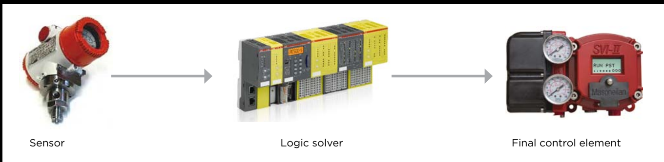
Figure 2. At its simplest, a safety instrumented system consists of a sensor, a logic solver (controller) and final control element.
