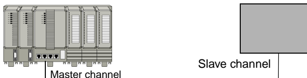
Figure 27. Master/slave in a point-to-point communication configuration.
