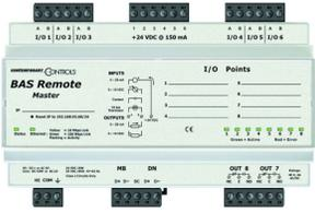
**2A-CC:** Very basic Tier 2A controller capable of monitoring six analog inputs and reporting their values to the network and setting two outputs. Network is BACnet over IP over 10/100 Mbps.
