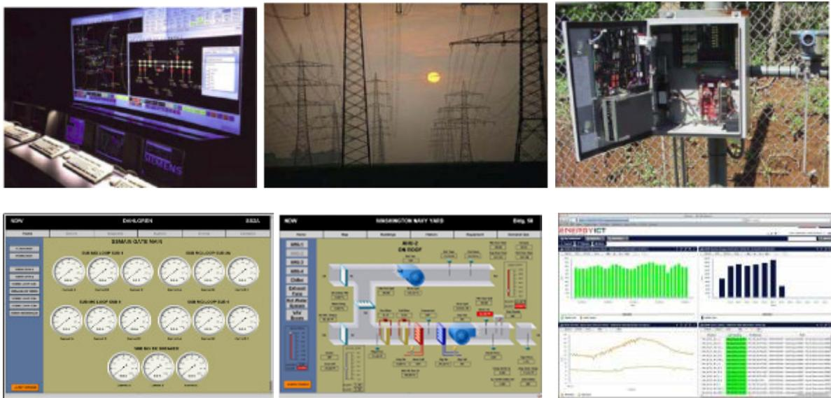
**Figure 1 – ICS Human Machine Interface, System, Remote Terminal Unit<sup>38</sup>**
