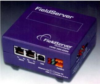
**2C-FS:** A Tier 2C gateway (application layer proxy). The Tier 2 network is Modbus over IP over 10/100 Mbps Ethernet. The Tier 1 network is proprietary over proprietary 2-wire media.
