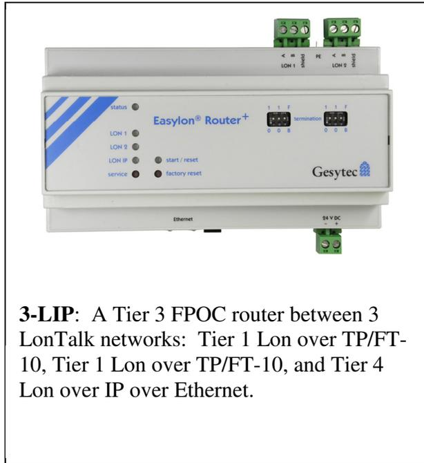
**Figure 6 – Tier 3: Facility Points of Connection (FPOCs)**
