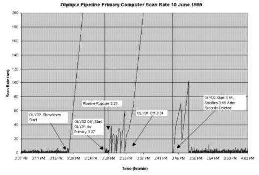
Figure 3. SCADA Response
