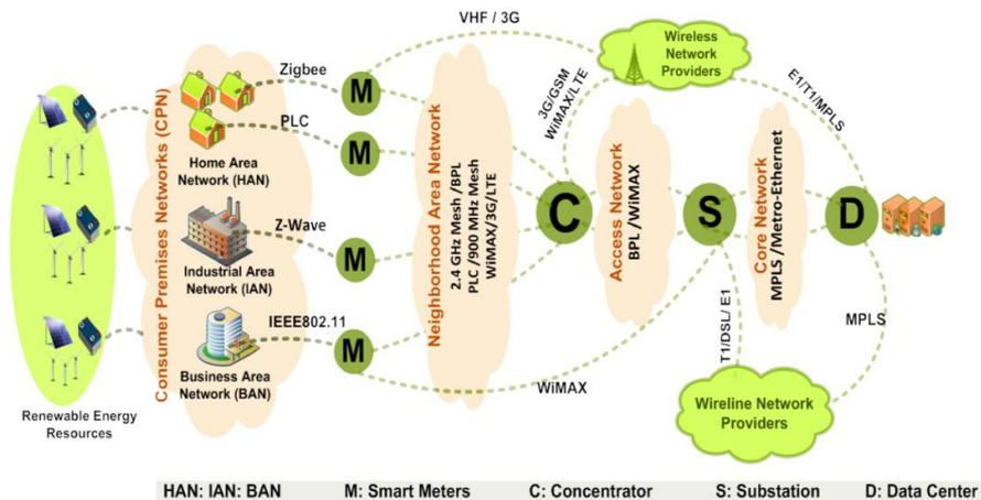
Figure 3: Basic network architecture<sup>4</sup>.
