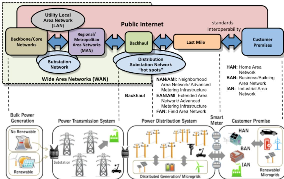
Figure 2 shows an overview of the standard communications architecture of a smart grid. This scenario considers the communications making use of the Internet due to the physical separation between the different sites of each section.
